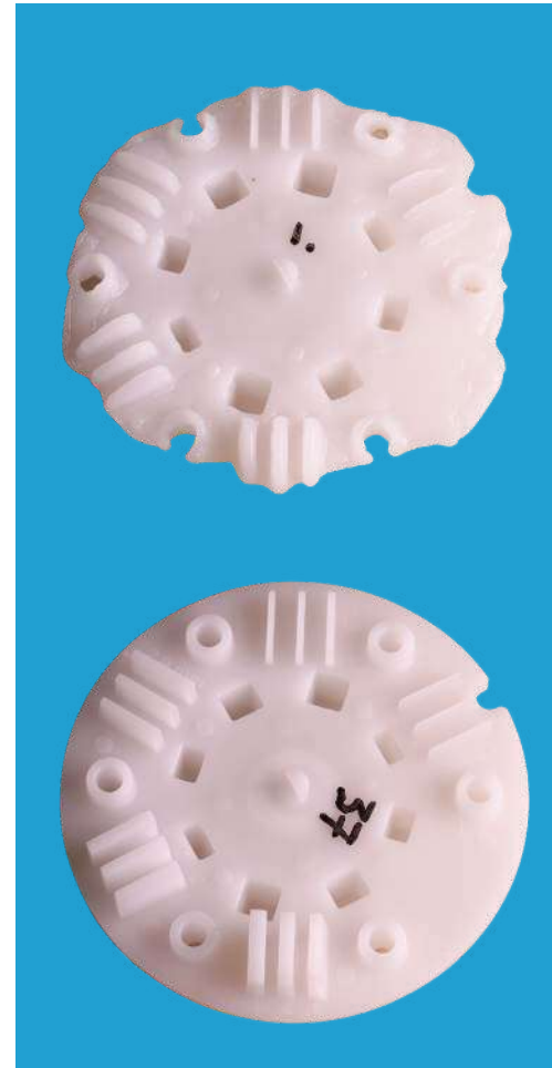
Shot 1 (top, start up, incomplete fill), and shot 37 (POM). Images © DREIGEIST
