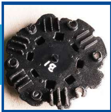
Molded part A, the intact tool had 1.5 minutes of IPA contact
