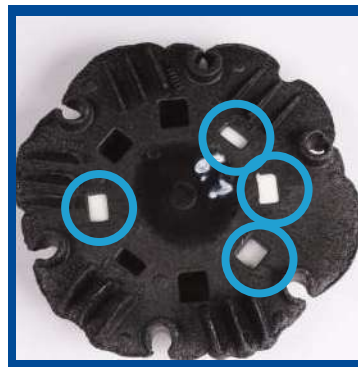
Molded part B, the broken tool had 5 minutes of IPA contact
