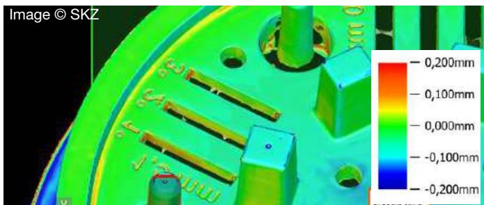
Comparison of tool and CAD file via surface topography
